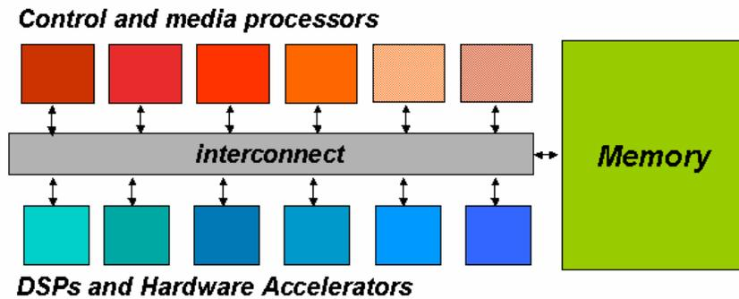
Figure 4-2. Heterogeneous SoC architecture with CPUs, DSPs, and accelerators communicating through shared memory.
