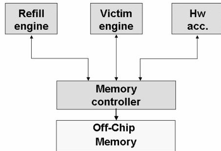
*Figure 4-11.* Memory controller ports.
