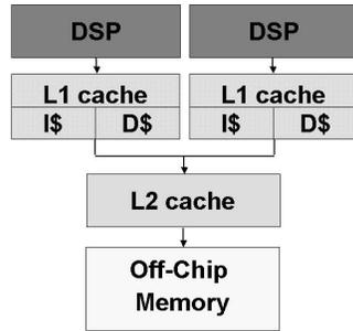
Figure 4-3. Data path for the memory hierarchy.
