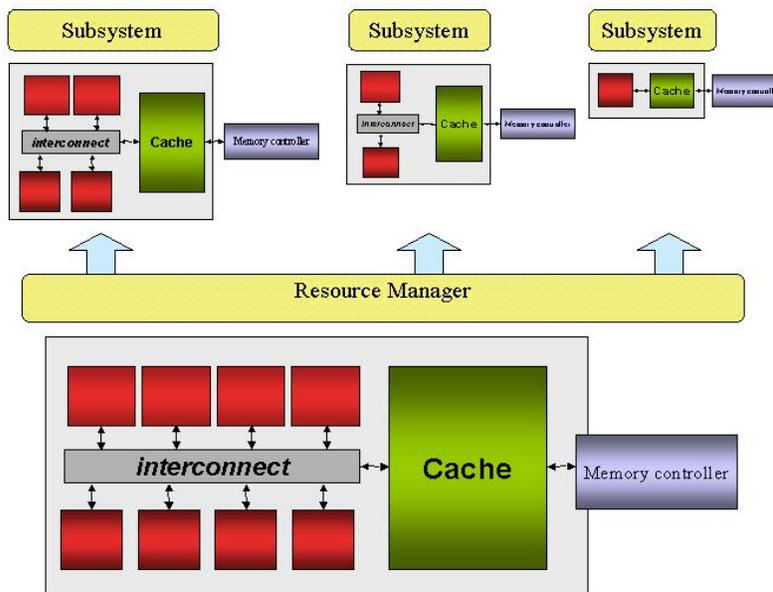
Figure 4-6. Providing virtual platforms to subsystems.
