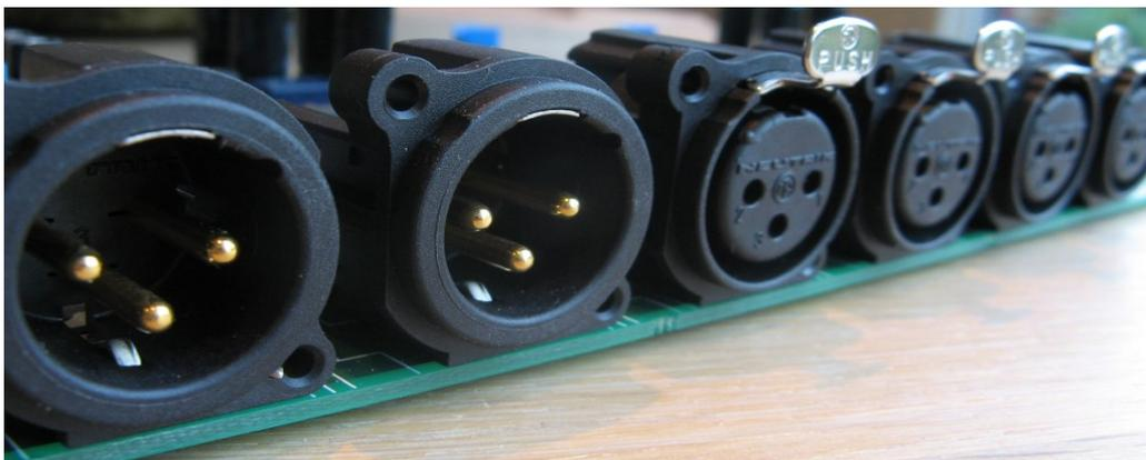
If you want to equip the preamp with 3 pair of XLR inputs plus 3 pair cinch inputs, diode D4D should NOT be mounted. Alternatively, if you want 2 XLR inputs and 4 cinch inputs, do insert D4D, and connect the 4<sup>th</sup> cinch pair to the pins marked with '+' on J4L and J4R. As in the regular use of XLR connectors for audio, the output connectors are 'male' (have pins), and the input connectors are 'female' (have holes).
