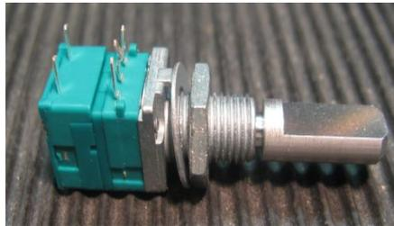
Type A, produced by DDM, is Conrad art.nr. 705594-89, which I have used for a long time already, and for which the PCB footprint was designed. It lacks a facility to screw it into a front plate. I only recently discovered type B in the Conrad catalog, art.nr. 700697-89. This switch from Alps (type STEC11B03) seems a better choice: its clicks feel smoother, and the metal housing and shaft have a better fit, more suitable for heavy control knobs.
