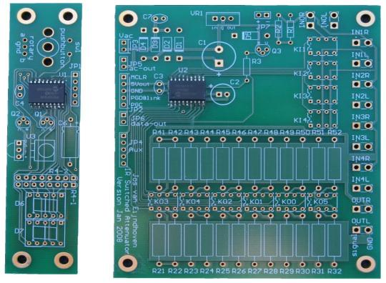
All required (PCB-mount) components are provided seperately, for your own mounting&soldering. Choose a mounting sequence with the lowest profile components first. That allows easy fixing of the components while PCB lies upside-down on your desk.
